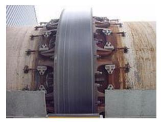
Tyres, sometimes called riding rings, usually consist of a single annular steel casting, machined to a smooth cylindrical surface, which attach loosely to the kiln shell through a variety of "chair"
