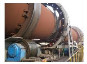
A rotary kiln is a pyroprocessing device used to raise materials to a high temperature (calcination) in a continuous process. **Materials** produced using rotary kilns include:
