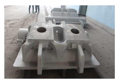
Roller cover is an important part mill. coal It is assembled with bearing block and grinder mill through the support of roller
