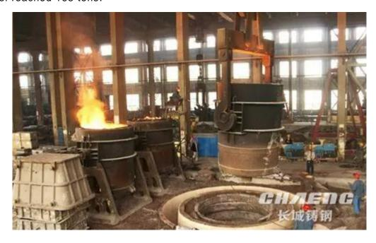
At the end of February 2016, the three-ladle pouring method was used to successfully cast the 88-ton press machine body. The actual amount of molten steel smelted this time reached 129 tons.
