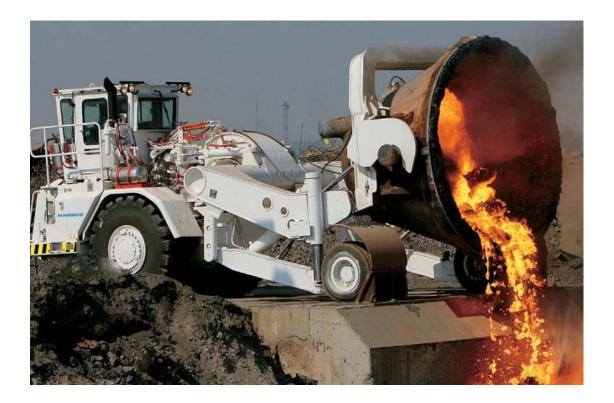
In order to ease the contradiction between steel slag transportation and the development of steel mills equipment technology of domestic, the GW90 slag pot carrier has been designed and developed.
