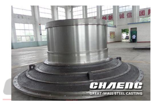
CHAENG is one of the large steel casting plants in China, specializing in processing large steel castings of various materials, among which the ball mill head is one of the star products of CHAENG.
