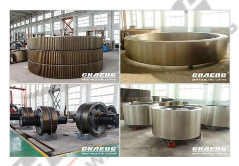
Main steel casting parts for ball mill: girth gear, mill trunnion, mill hear, bearing housing, etc.
