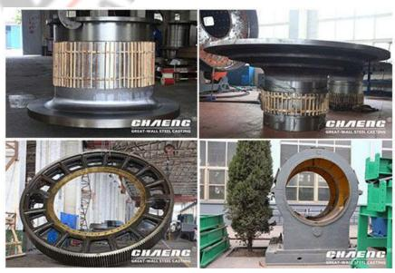
Main steel casting parts for vertical roller mill: grinding roller, grinding table, rocker arm, bearing chock, etc.
