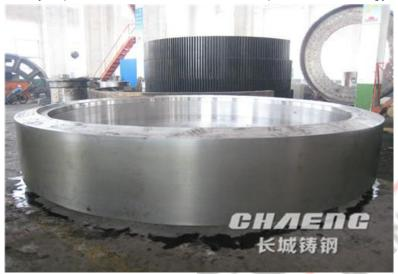
CHAENG (Great Wall Steel Casting) is a steel casting factory established in 2007 and has good and stable cooperation with many companies in the cement industry. The casting tyre for rotary kiln have high hardness, good crack resistance, and strong abrasion resistance.
