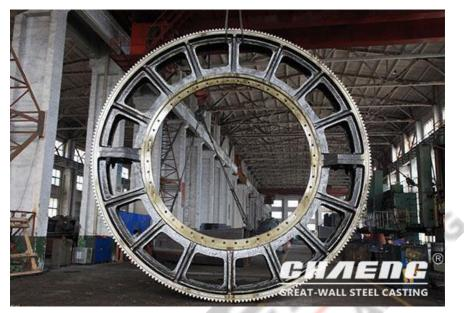
The girth gear requires high hardness and wear resistance of the tooth surface, and sufficient toughness of the tooth core. And the girth gear with complex shape and large diameter usually adopts carbon steel and alloy steel with carbon content of about 1.4% to ensure the quality, so ZG35Mn, ZG35CrMo, ZG42CrMo are often used. The following are the composition of ZG35Mn, ZG35CrMo, ZG42CrMo:
