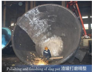
Polishing and finishing of slag pot 渣罐打磨精整
