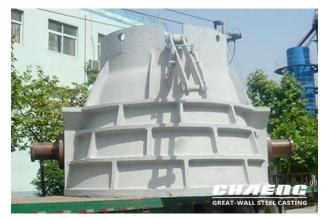
Slag pots are important equipment for steelmaking in the metallurgical industry, and their quality directly affects production. Large steel mills usually purchase large slag pots above 10m<sup>3</sup>, which are relatively difficult to control because of their large size.
