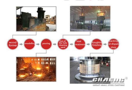
Base on the requirements of customers, CHAENG selects appropriate wooden mold for modeling design, and uses CAE software to simulate the casting process. Strictly according to the process procedures to produce high-quality ball mill trunnion: wood mold - modelling - pouring - heat preservation - out of
