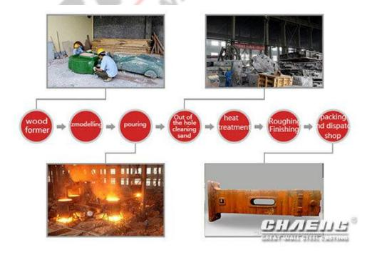
Base on the requirements of customers, CHAENG selects appropriate wooden mold for modeling design, and uses CAE software to simulate the casting process. Strictly according to the process procedures to produce high-quality press frame: wood mold - modelling - pouring - heat preservation - out of the pit, sand cleaning - heat treatment - roughing, finishing - packing and delivery.
